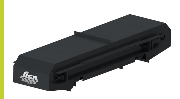
The overband magnet is placed over a belt conveyor. The permanent magnet removes ferrous particles from the material flow passing underneath it and drops the ferrous particles into a tray or container next to the underlying conveyor.
