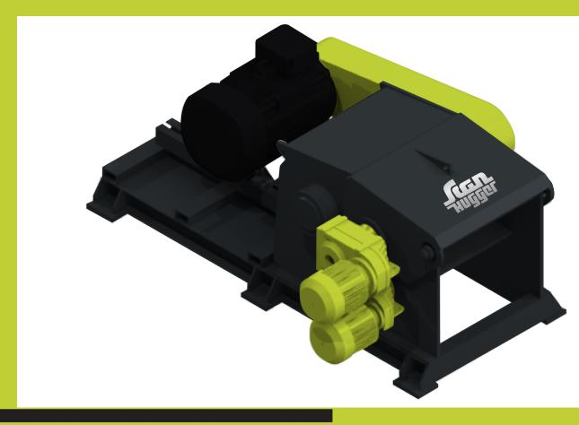
The Scanhugger HT 75/60/4 wood chipper is mounted with a solid steel drum rotor designed to produce the requested chip size. The straight knives are mounted with a special wedge system that lock and secure the knives in the rotor. This system is ideal for shredding short or long lengths of solid waste wood, from the timber sizing and wood processing industry in order to produce a defined homogeneous wood chip.
