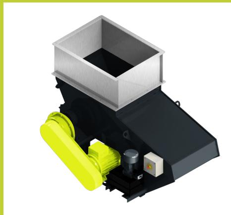
Scanhugger HL 4/18/30 is an all-round shredder capable of shredding up to 6000 kg/hour. The shredder is designed all types of wood waste, ranging from hard- and softwood, trim blocks, particleboard, MDF, furniture parts, paper, and cardboard. Depending on the desired chip quality, the machine can be mounted with two different rotor types and various screen sizes.
